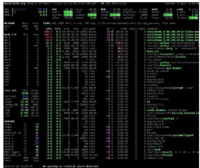
Figure 4: The glances interface with network, disk, filesystem, and sensor information.
